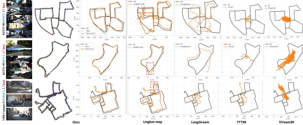
Figure 4: Qualitative comparison on long-sequence 3D reconstruction. As sequence length grows, existing methods show pose degradation, drift, or collapse. Lingbot-map exhibits progressively stronger pose jitter over longer rollouts, while HorizonStream maintains stable pose estimation.
